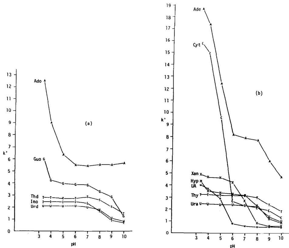
Fig. 2. Effect of pH on the capacity factors of (a) nucleosides and (b) bases. Column, 9- $\mu\text{m}$  Asahipak GS 320H; mobile phase, 0.01 M SDS; flow-rate, 2 ml/min; temperature, ambient. Each point represents the average of three determinations.
