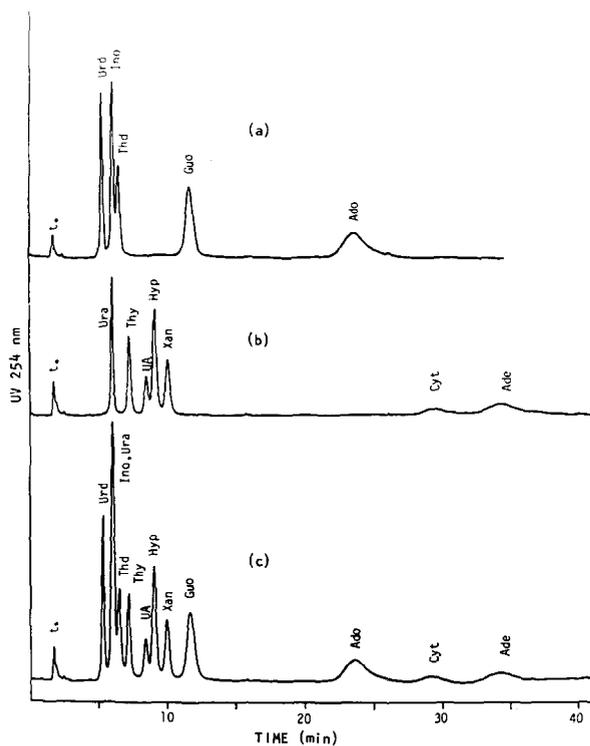
Fig. 1. Isocratic elution profiles of (a) nucleosides, (b) bases, and (c) a mixture of nucleosides and bases. Column, 9- $\mu\text{m}$  Asahipak GS 320H; mobile phase, 0.01  $M$  SDS (pH 3.4); flow-rate, 2 ml/min; sample concentration,  $2 \cdot 10^{-5}$   $M$  each; injection volume, 10  $\mu\text{l}$ ; sensitivity, 0.01 a.u.f.s.; temperature, ambient.
