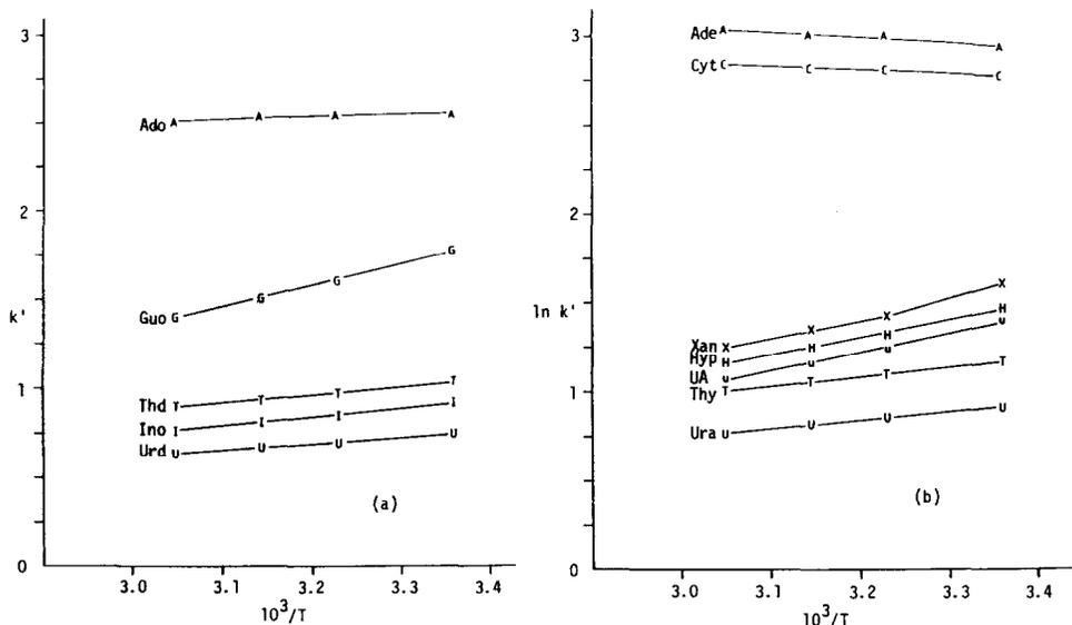
Fig. 7. Van 't Hoff plots of the capacity factors of (a) nucleosides and (b) bases. Temperature, 25, 37, 45 and 55°C; mobile phase, 0.01 M SDS (pH 3.4); flow-rate, 2 ml/min. Each point represents the average of three determinations.
