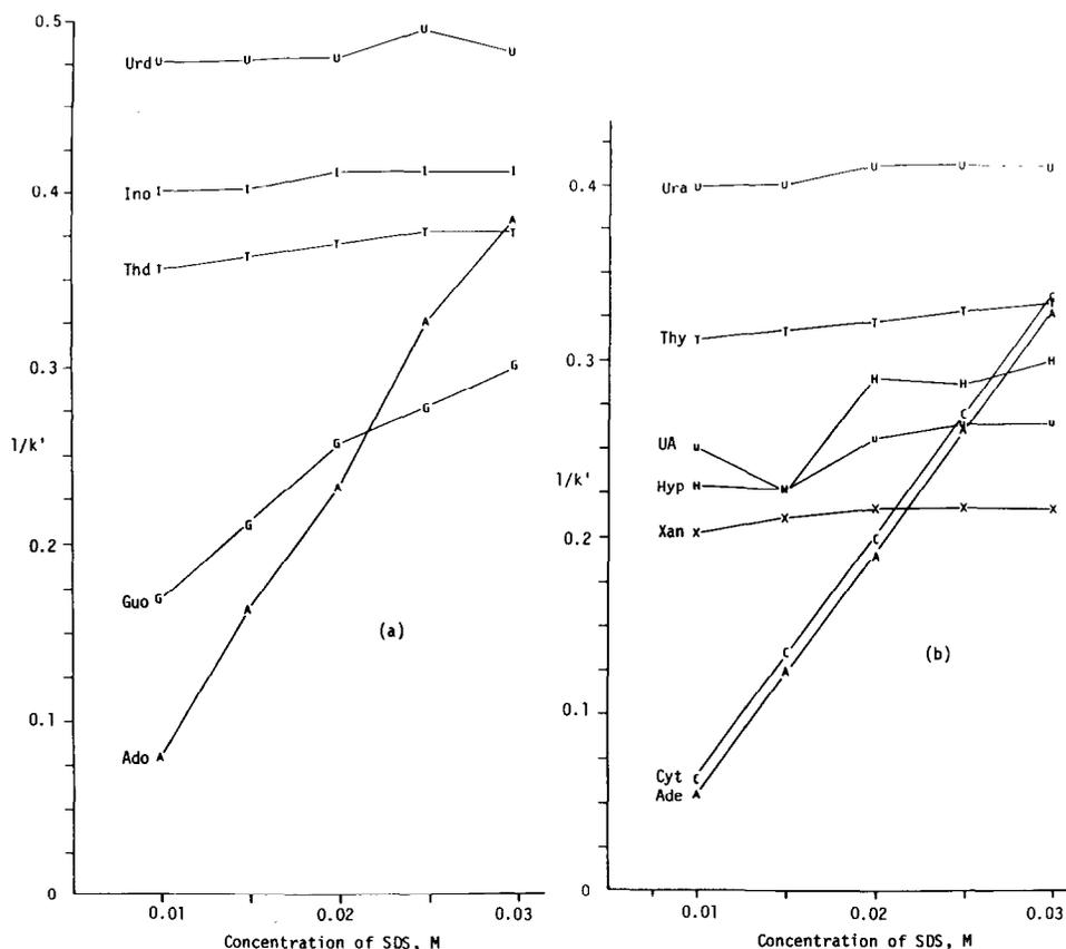
Fig. 5. A plot of SDS concentration against the reciprocal of the capacity factors of (a) nucleosides and (b) bases. All chromatographic conditions are the same as in Fig. 4. Each point represents the average of three determinations.
